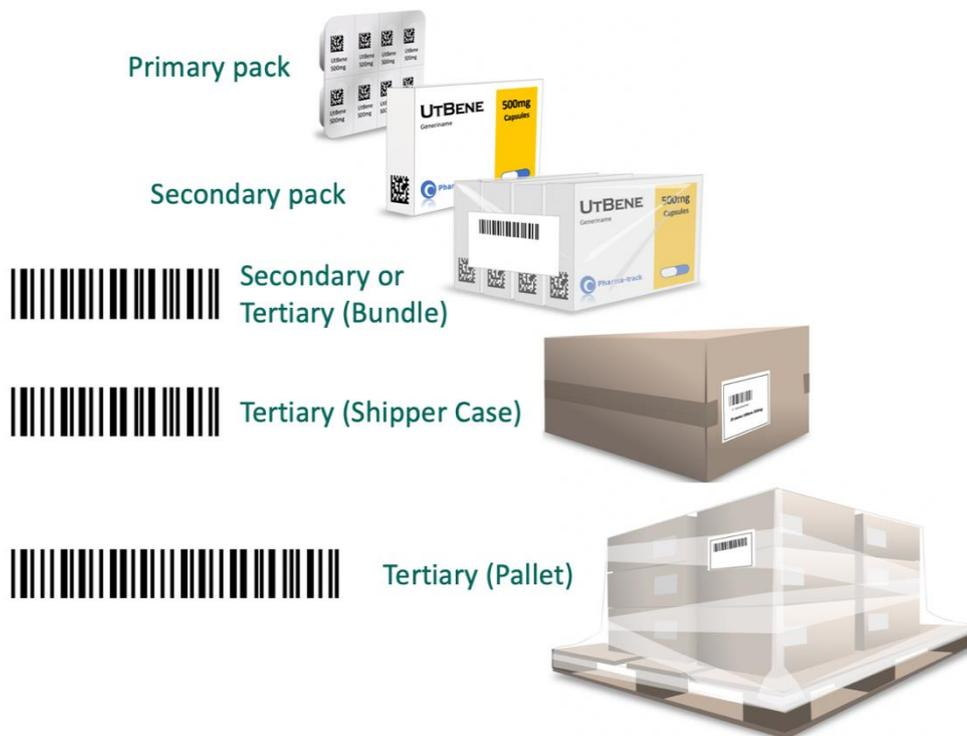
**Figure 14: Packaging hierarchy, aggregation, and associated codes**
